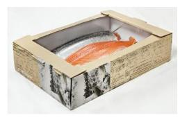
In 2015, the S Group tested a **new fibre-based packaging solution** for fish products to replace the traditional Styrofoam boxes. Renewable wood fibre is used to make the EcoFishBox. It is waterproof and leak tight because of a thin PET-film that is pre-laminated on the liner and the special way of the packaging is folded. When tested by the S Group, it was found that **the fibre-based box performed well in the logistics chain,** as well as being
